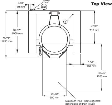
= Electrical connection CWI = Cold Water inlet 1" CWO = Cooling Water Outlet 1"
